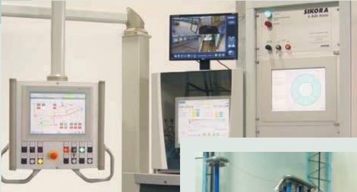
Finolex CCV (Continuous Catenary Vulcanisation) line is equipped with most modern new generation X-Ray type diameter controller for measuring, monitoring and controlling of thickness, diameter and eccentricity throughout the length.
